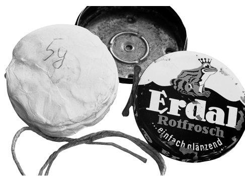
Figure 4. Shoe polish can used as a reaction vessel for the manufacture of styropor®.
